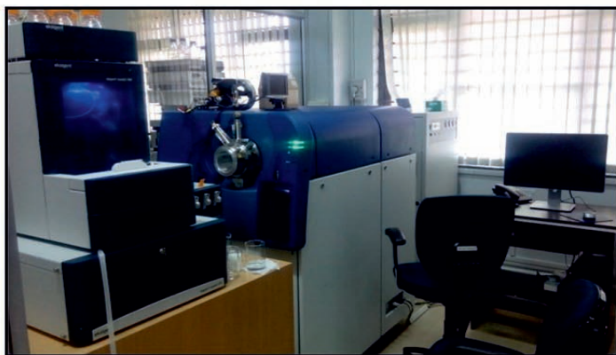
nLC-ESI-Q-TOF, Model: 5600 Plus, SCIEX, USA
