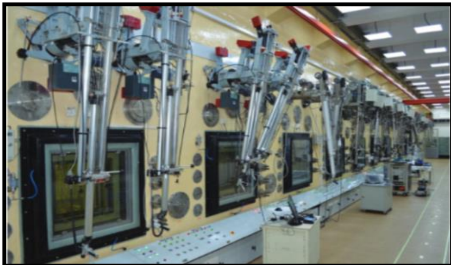
Hot cell facility at BARC for handling radioactive samples
